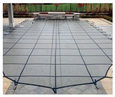
INVIS-A-DRAIN - The Invis-A-Drain is constructed with 1/4" drain holes placed every 6" in reinforced vinyl down the center of the cover. Beneath is a 12" wide mesh drain panel designed to allow water to drain through while filtering out small debris. Invis-A-Drain comes standard on all custom Hyperlite covers.
